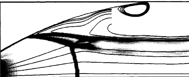
Fig. 16 Schlieren-type snapshot and instantaneous streamlines for the case of PR = 30 .
